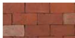
Clay paving bricks differ from the brick used on walls and chimneys, in that paving bricks are solid, without holes. (See pg.16 for cored brick) In addition, paving bricks are fired to a different standard than face bricks to insure long-term durability. Our clay pavers come in a "flashed" color which means there are a variety of red and brown shades mixed on the pallets.
